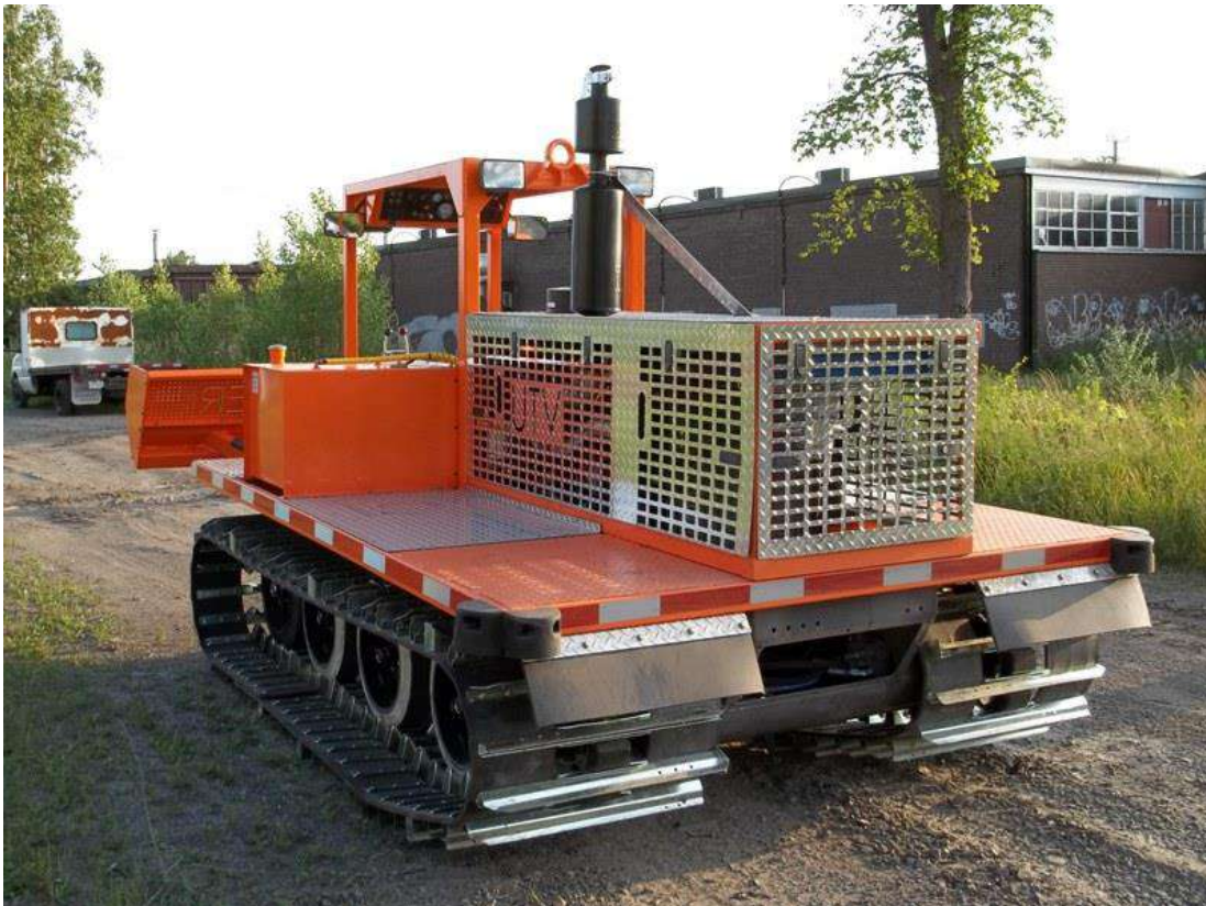
RT-01 U Ship Trimmer with 28.5" hardened steel crosslinks & 2 way Heavy Duty Straight Blade
