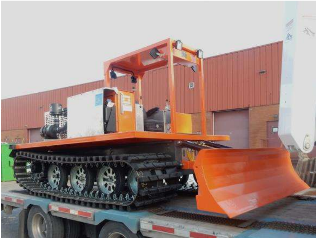
RT-01 U Ship Trimmer with 29" Rubber Tracks & 2 way Heavy Duty Curved Blade
