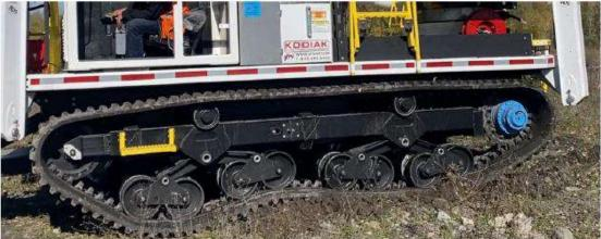
Full ground contact of the track system for a higher, mobile full traction.
