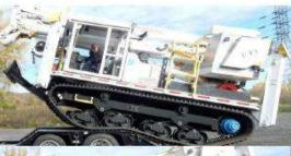
As shown in the images to the left, the Patented Double Walking Beam system ensures the track is always making maximum contact with the ramp, thus reducing the vehicle pitch when climbing over it.
