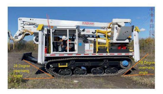
High overhang angle facilitates crossing over ditches and high obstacles.
