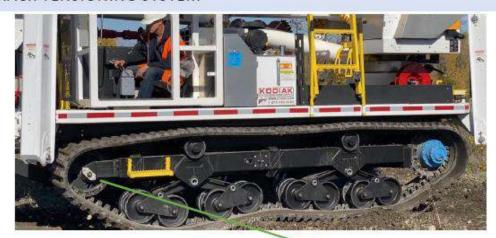
Automatic track tension and length compensation system: Grease filled cylinders and volute springs
